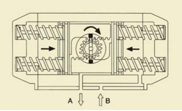
In the event of loss air pressure or power, the stored energy in the springs forces the pistons inwards, Rausing the pinion turns clockwise while air is being exhausted from Port A, and air to Port B can accelerate closing the valve.
