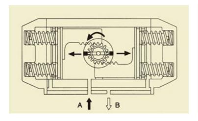
Air into Port A forces the pistons outwards, causing the springs to compress, the pinion turns counterclockwise while air is being exhausted from Port B.
